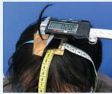
damage the individual fibres. The LED screen of the digital vernier caliper will display the hair mass in millimetres. This indicates thickness in millimetres of hair in a 20×20mm<sup>2</sup> area of the scalp examination zone.
